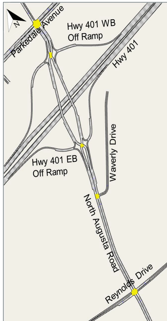
Figure 56: North Augusta - Diverging Diamond Configuration
